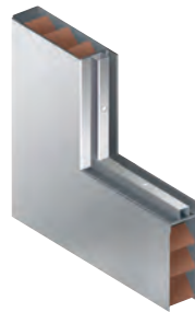
DLF flush vision kit , 16-gauge (0.056”/1.4 mm). Laser welded, available for 1/4” (6.3 mm) to 1” (25.4 mm) thick glass (FK series).
