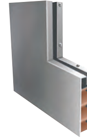
DLF flush seamless vision kit , 16-gauge (0.056”/1.4 mm). Laser welded, available for 1/4” (6.3 mm) to 1” (25.4 mm) thick glass (FKS series).
