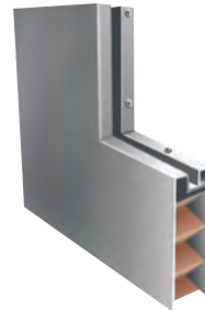
DLF flush seamless vision kit , 16-gauge (0.056”/1.4 mm). Laser welded, available for 1/4” (6.3 mm) to 1” (25.4 mm) thick glass (FKS series).
