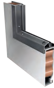
Standard two-part sandwich-type vision kit, welded corner sections , 18-gauge (0.044”/1.1 mm). Available for 1/4” (6.3 mm) to 1” (25.4 mm) thick glass (SK series).
