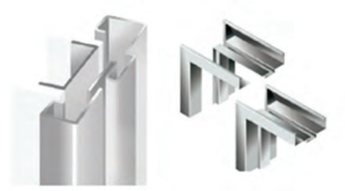
Split frame wrapping steel stud with drywall.
