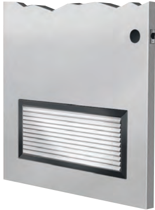
Standard two-part sandwich-type louver , inverted “Y” blades, welded corners, 50% free-flow area, 18-gauge (0.044”/1.1 mm).
